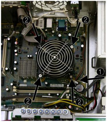
When reinstalling the heat sink, make sure that its bottom has been cleaned with an alcohol wipe and fresh thermal grease has been applied to the top of the processor.
